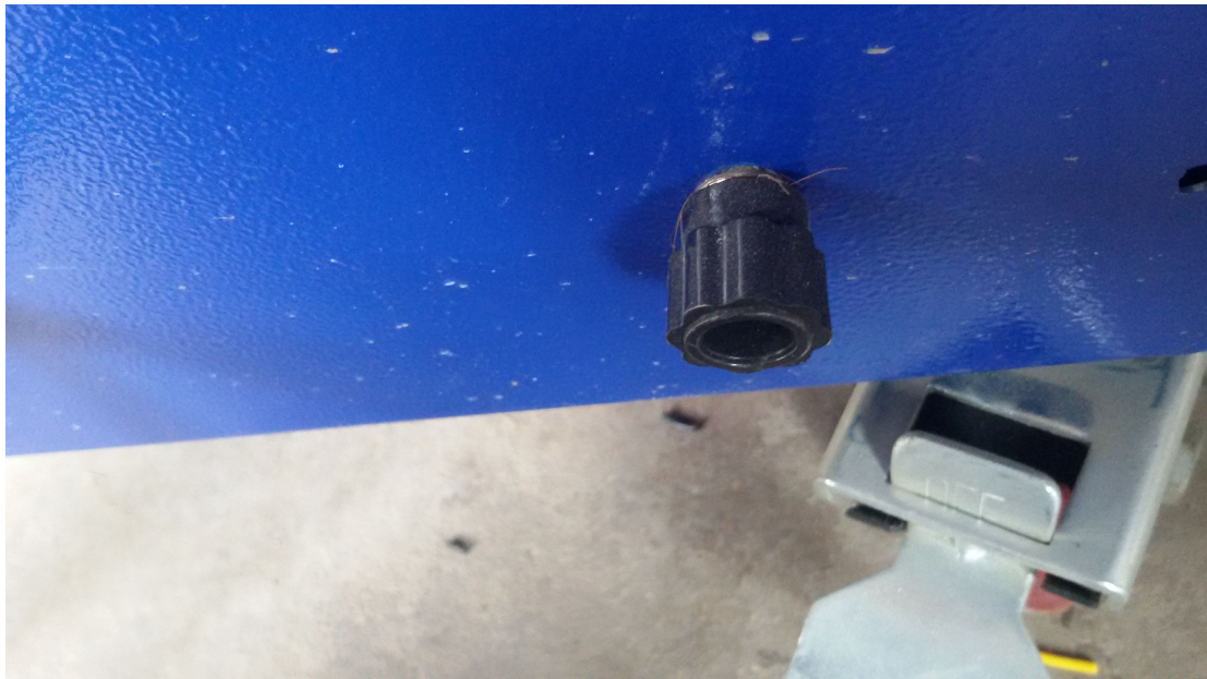
Picture A-15 earth wires connection port
